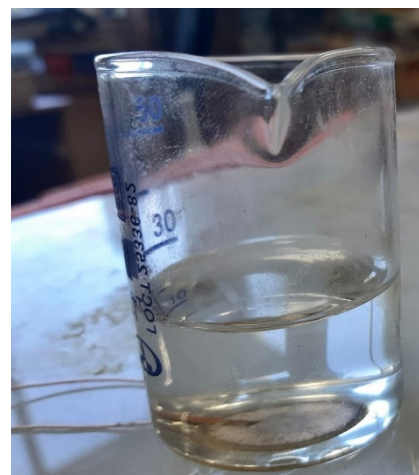
Fig. 1. Standard laboratory glass with piezoelement glued to the bottom
